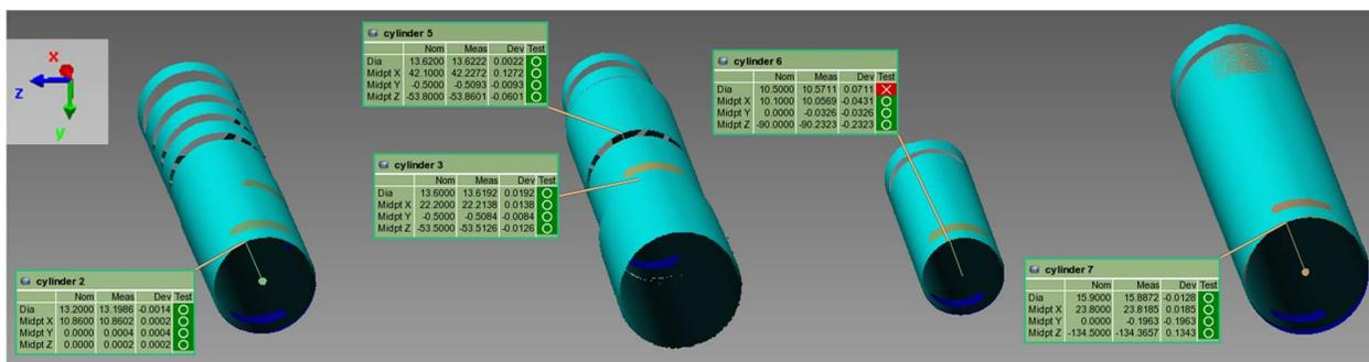
**Figure 5:** Four bores in a valve body were scanned and analyzed in one inspection sequence. The results include dimensional measurements and pass/fail reporting for each bore, as well as the bore pitch (bore spacing), and exact positioning of each bore on the valve body.
