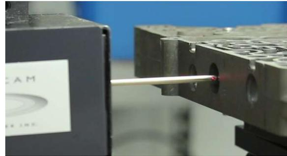
**Figure 1:** The optical probe of the BoreInspect scans a valve-body bore ID as it is rotated and moved into the bore
