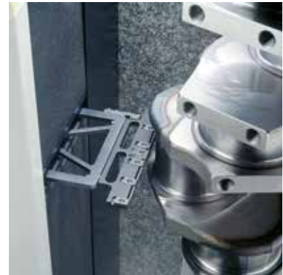
Flat measuring follower for crankshafts
