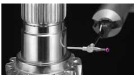
Twist measurement with a roughness stylus tip
