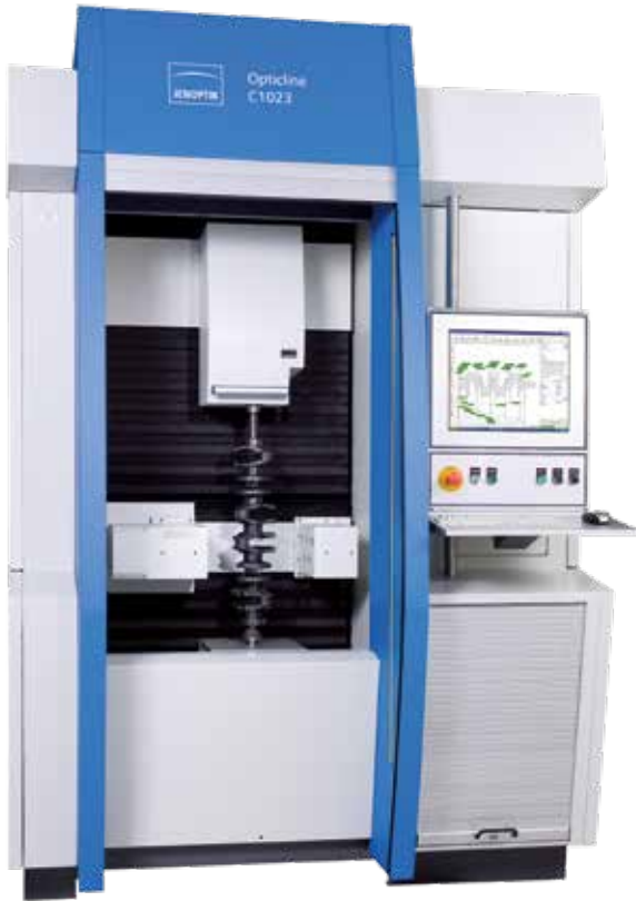
Opticline C1023 with safety light barrier and roller shutter
