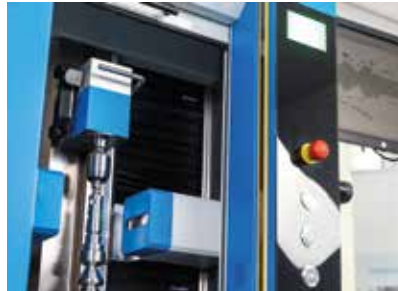
Integrated light barrier to protect operators in accordance with international safety standards
