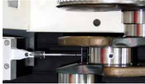
Optional tactile probing system BTS for concentric lengths and axial run-outs
