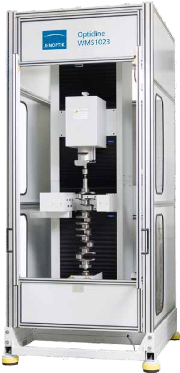
Opticline WMS1023 in a vertical design
