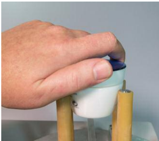
Anditork , for manual torque measurements on closures
