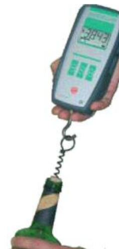
Extractor , for the manual measurement of the extraction force on corks
