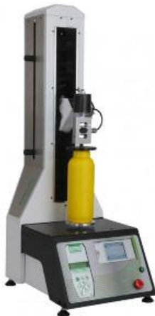
Topload , for automated crush tests on bottles
