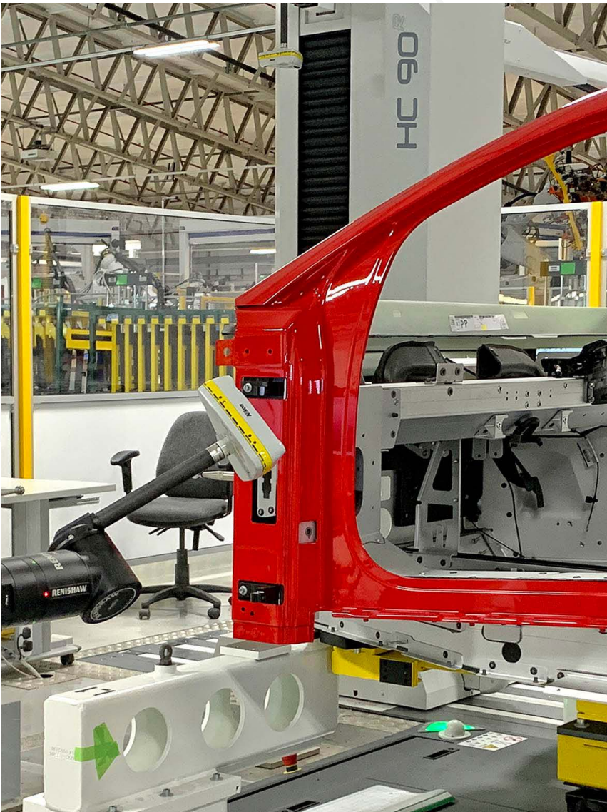
A Renishaw PHS-2 wrist (left) allows infinite positioning of the Nikon XC65DX-LS cross scanner, ensuring that the required inspection data is acquired on the LK CMM well within the TAKT time of the Emira production line.
