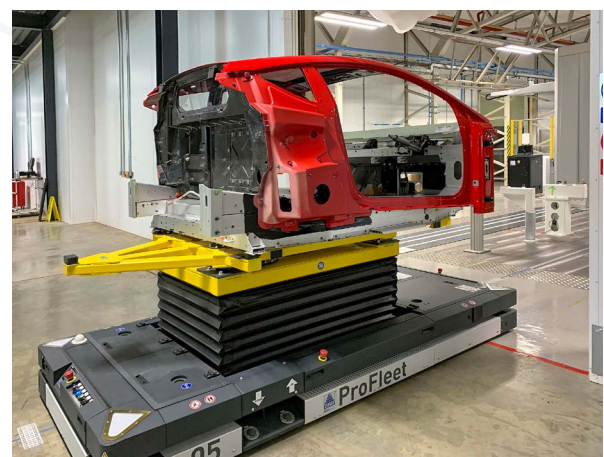
A Lotus Emira being delivered by an automated guided vehicle from the production line to the LK CMM to undergo stage 1 inspection.
