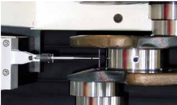
Probing system BTS for Opticline C1000, AMV and WMS
