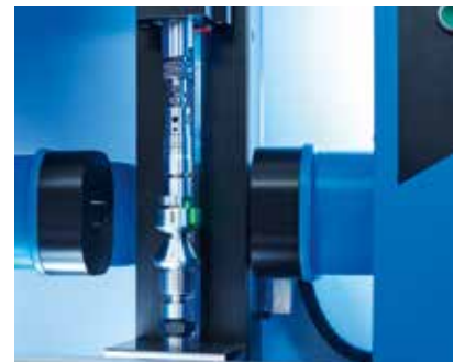
Simple clamping of the workpiece between tips
